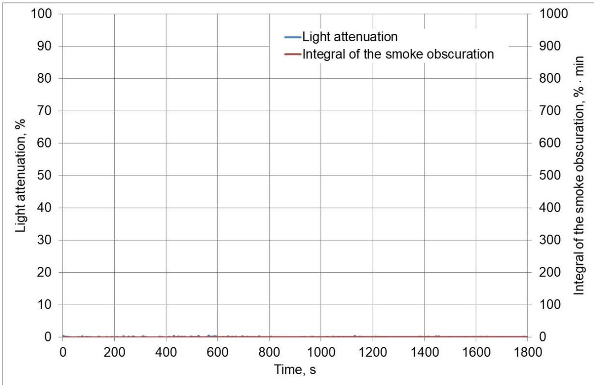
Fig. 3. Smoke generation during the test - specimen 3
