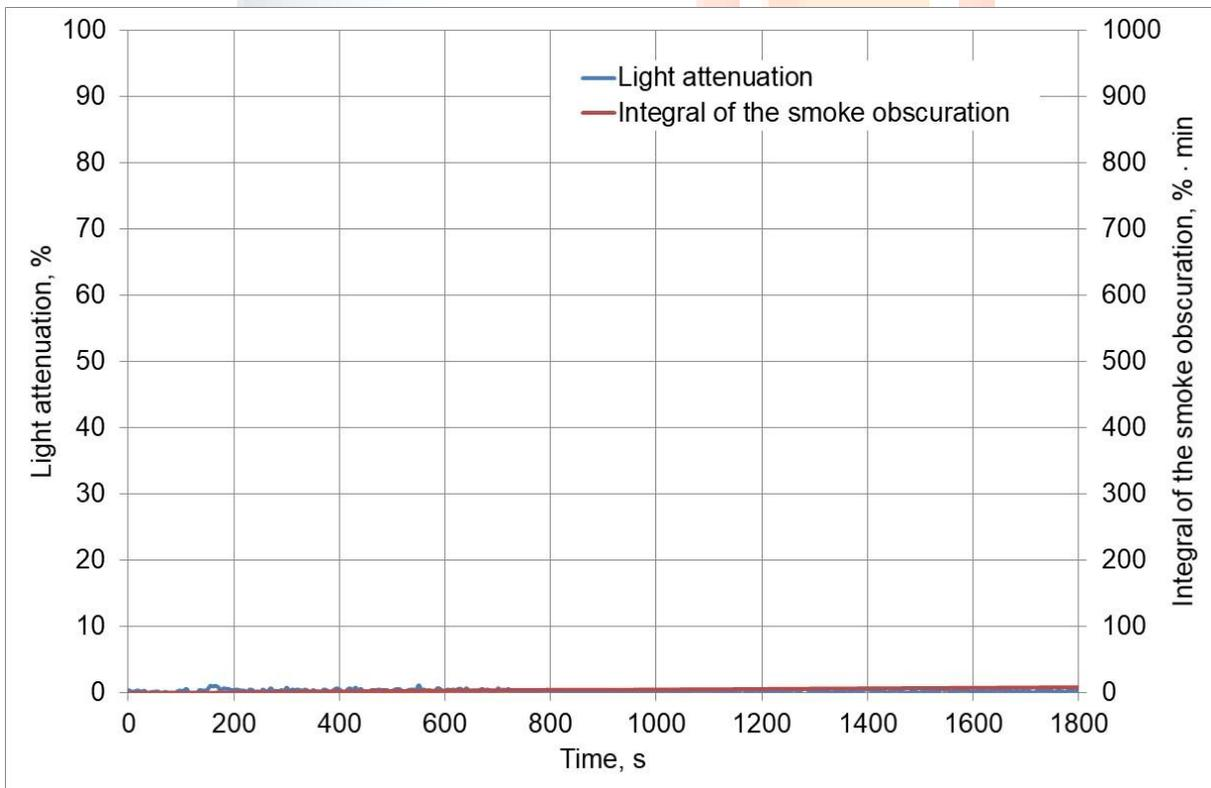
Fig. 2. Smoke generation during the test - specimen 2
